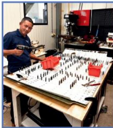
Martinus moving the rivet holes from the old skin to the new skin.
