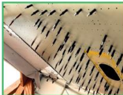
The new skin fits well, with all holes correctly positioned. We'll trim the overlapping yellow section for better access to the main gear.
